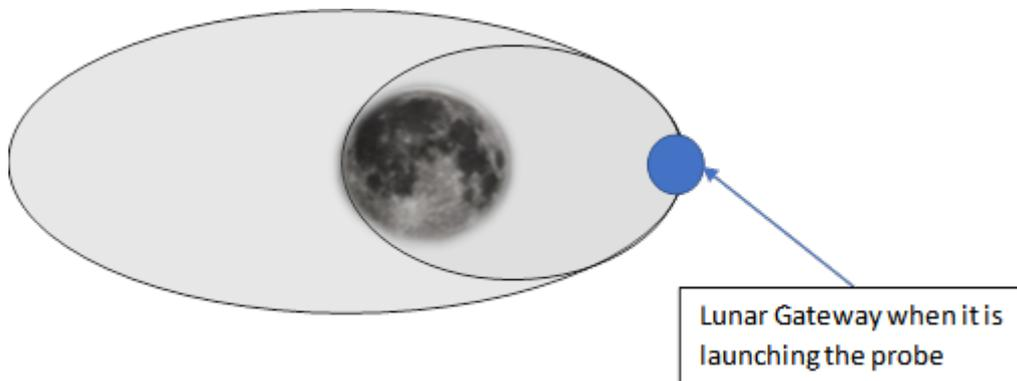
**Figure 2:** Illustration of the orbits of LOP-G and the probe, before and after the change in the probe’s orbit.
